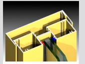
Can accept both captive and roll-in wedges for the ease of site glazing. We can use silicone wet top on the outside in lieu of the captive wedge.
